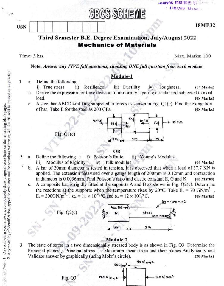
The state of stress in a two dimensionally stressed body is as shown in Fig. Q3. Determine the 3 Principal planes, Principal stress, Maximum shear stress and their planes Analytically and Validate answer by graphically (using Mohr's circle). (20 Marks)
